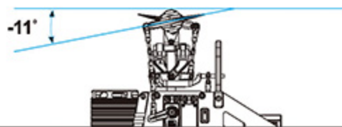
Stick Position at Low/Throttle 100%/Pitch -11° 搖桿低速/油門100%/Pitch -11°
