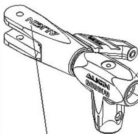
Feathering shaft 橫軸 φ6×φ8×93.2mm
