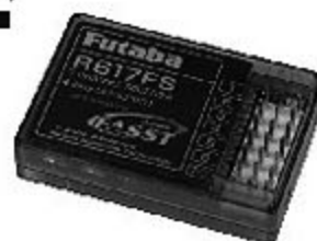
Receiver (6-channel or more) 接收機(七動以上)
