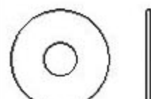
Washer 橫軸墊圈 (φ4×φ12×1mm)x2
