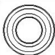
Bearing 軸承 (φ10xφ19x5 mm) x2
