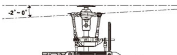
Stick position at low/Throttle 0%/Pitch-2°~0° 搖桿低速/油門0%/Pitch-2°~0°
