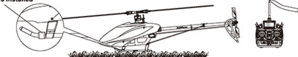
Rubber skid stoppers installed 裝上避震墊圈
