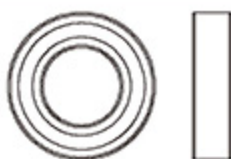
Bearing 軸承 (φ 10x φ 19x5mm) x 2
