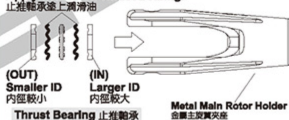
Feathering Shaft Sleeve 橫軸支撐套 φ8xφ10x31mm
