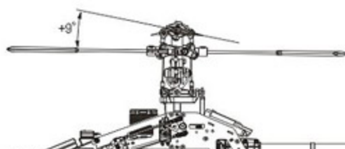
Slick position at high/Throttle 100%/Pitch +9° 搖桿高速/油門100%/Pitch+9°
