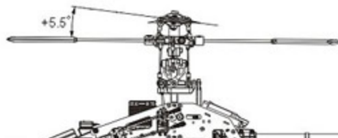
Slick position at Hovering/Throttle 70%/Pitch +5.5° 搖桿停懸/油門70%/Pitch+5.5°
