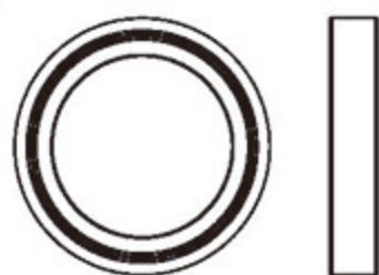
Bearing 軸承 (φ 15x φ 21x4mm) x 2
