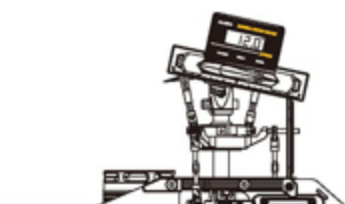
Stick Position at High/Throttle 100%/Pitch+12° 搖桿高速/油門100%/Pitch+12°
