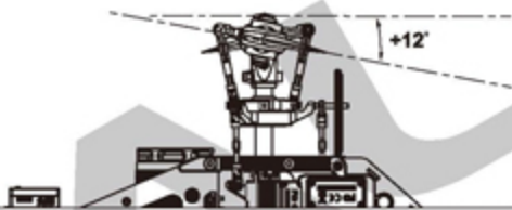
Stick Position at High/Throttle 100%/Pitch+12° 搖桿高速/油門100%/Pitch+12°
