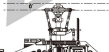
Stick Position at Middle/Throttle 90%/Pitch 0° 搖桿中速/油門90%/Pitch 0°
