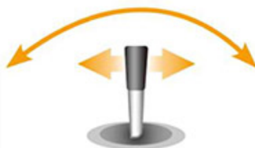
Tap aileron stick to swap colors 輕推副翼搖桿反向設定燈號
