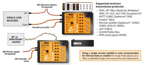
Always make sure the power supply is stable and dimensioned sufficiently for the intended application. If possible always connect the power source directly to MICROBEAST PLUS (not at port [AUX|PIT|RUD]) but additional supply cables can be plugged into free receiver ports, too. Especially when using standard size servos it is recommended to use more than one power supply cable in parallel to preserve a stable voltage and to reduce power loss due to connection resistance.
