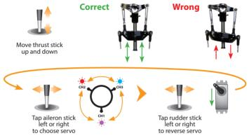
After adjusting servo directions make sure that the pitch direction is correct! You can either do this by setting the servo directions correctly right from the beginning or by changing the direction of the pitch channel in the transmitter later.
