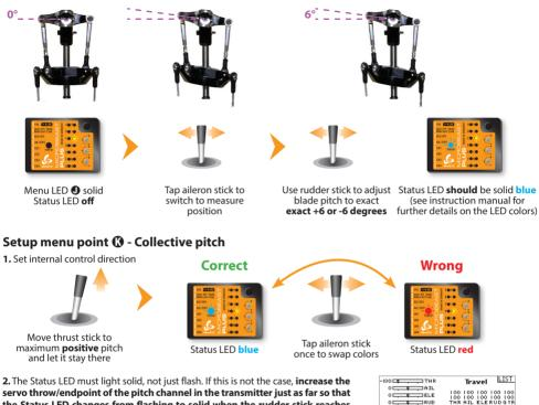
the Status LED changes from flashing to solid when the rudder stick reaches the end position. But do not increase the endpoint too much in the transmitter! We need an exact match of full stick position and stick end position, the Status LED should just change from flashing to solid when reaching the end position.
