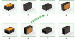
Use one of the supplied 3M gyro pads to stick the device to your helicopter. The device housing must not directly touch the chassis of the helicopter. When connecting and laying out the servo and receiver wiring later onwards please make sure the wires do not pass tension to the MICROBEAST PLUS. It is not recommended to bundle or tie down the leads close to the MICROBEAST PLUS device.
