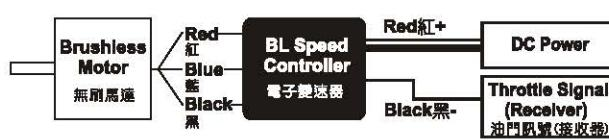
The motor rotates in different direction with different brand ESCs. If the wrong rotating direction happens, please switch any two cables to make the motor rotates in right direction.
