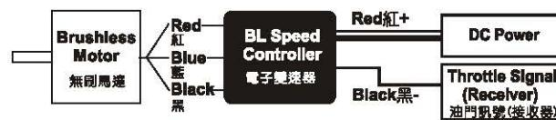
The motor rotates in different direction with different brand ESCs. If the wrong rotating direction happens, please switch any two cables to make the motor rotates in right direction.
